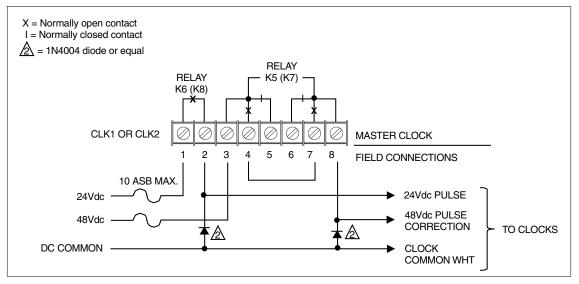
Figure B-20 Standard Electric Time AR-3 Three-Wire Impulse
